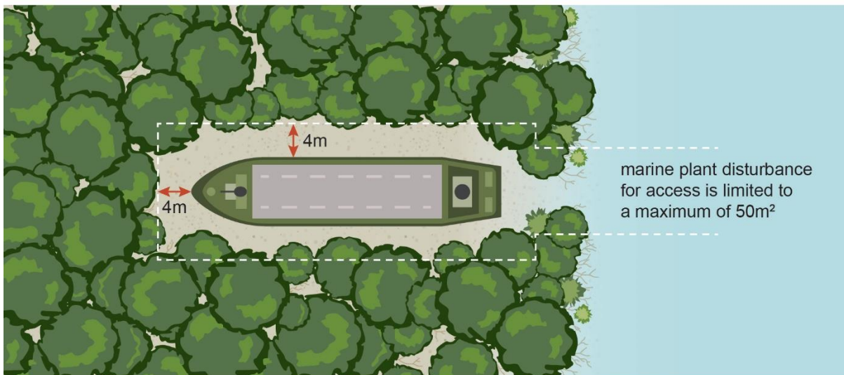
Figure 3: Removal of derelict vessels
