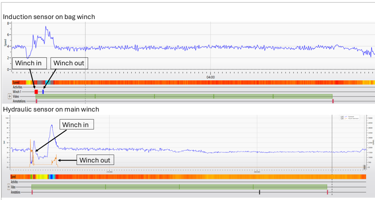
Figure 6: Example of winch in and winch out signals visible to the reviewer from an induction sensor on a bag winch and a hydraulic sensor on the main winch – for a vessel without sensors, only the blue line is available
